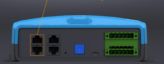
If it is the last device in the Bus, make sure to use a **RJ45 terminator** to end the bus
